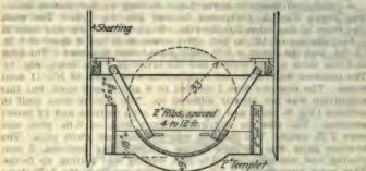
Fig. 20.—Concrete Sewer Construction.
